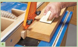
**Rout the first bevel** by standing each leg piece on edge, in a vertical position. Make a large push block, with a stop on the end, to hold the workpiece tight against the fence.
