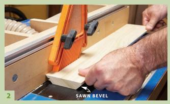
**Test the setup** by routing similar lock miters on two scrap pieces. Pre-cutting some of the bevel on the tablesaw produces a smoother profile.
