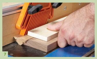
**Rout the second bevel** with the workpiece held horizontally. The jig provides a wide bearing surface in order to cut a perfect joint on this narrow piece.
