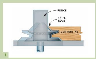
**Set up a lock miter** bit in your router table by aligning the center of the bit with the center of your material. Set the fence to produce a knife edge.
