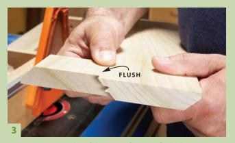
**Fit the pieces** together. If the top surfaces are flush, the setup is OK. If not, adjust the fence's position or the bit's height.
