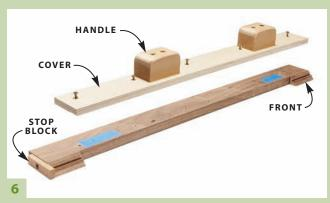
**Fasten a cover piece** to the jig and attach a stop block. Slide the workpiece into the jig from the front, with its lock miter engaged with the jig's profile.
