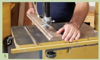
**Build a jig** for routing the second bevel. Rout a lock miter on this piece by standing it on edge, as in the last step. Remove the center portion of the lock miter profile using a bandsaw.
