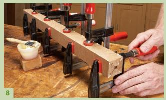
**Glue four identical pieces** to make the leg. The interlocking miters prevent the pieces from slipping side to side.
